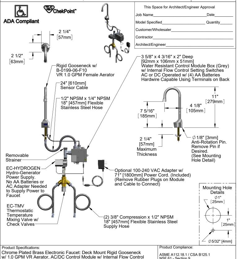
Setting Switches, Thermostatic Temperature Control Mixing Valve w/ Integral Check Valves, Hydro-Generator and 18" Flexible Stainless Steel Supply Hoses
