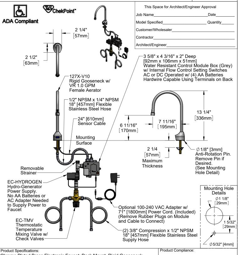
Chrome Plated Brass Electronic Faucet: Deck Mount, Rigid Gooseneck w/ VR 1.0 GPM Aerator, AC/DC Control Module w/ Internal Flow Control Setting Switches, Thermostatic Temperature Control Mixing Valve w/ Integral Check Valves, Hydro-Generator & 18" Flexible Stainless Steel Supply Hoses
