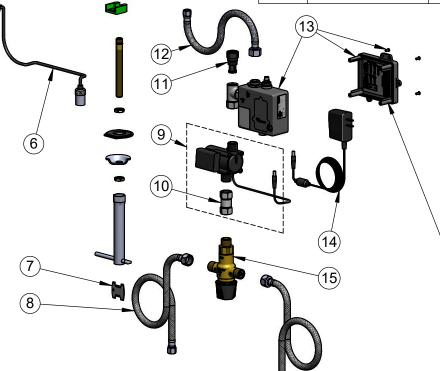
A Maximum of (8) ChekPoint Faucets can be Hardwire Connected and Powered by EC-HARDWIRE ChekPoint Hardwire AČ Transformer. (Sold Separately)
