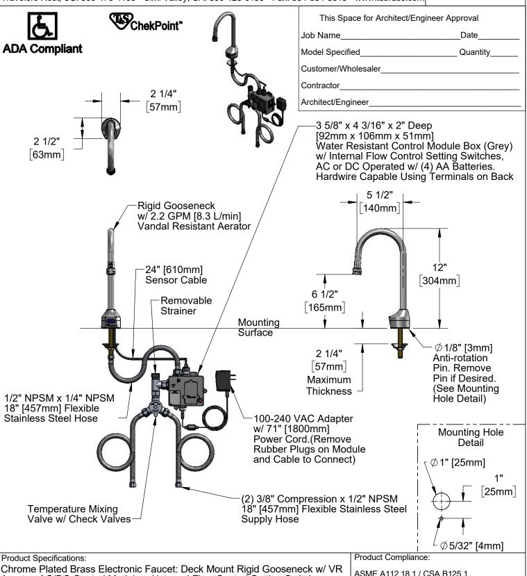
Chrome Plated Brass Electronic Faucet: Deck Mount Rigid Gooseneck w/ VR Aerator, AC/DC Control Module w/ Internal Flow Control Setting Switches, Temperature Control Mixing Valve, 18" Hot & Cold Supply Stop Flexible Connector Hoses
