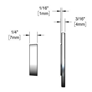
Note: The Plastic Deck Plate Spacer is Required for Secure Installation of B-0712 Series, B-2460 Series and Similar Faucets Installed with 013433-40 or 013434-40 Deck Plates. (See Installation with Deck Plate Detail Above)
