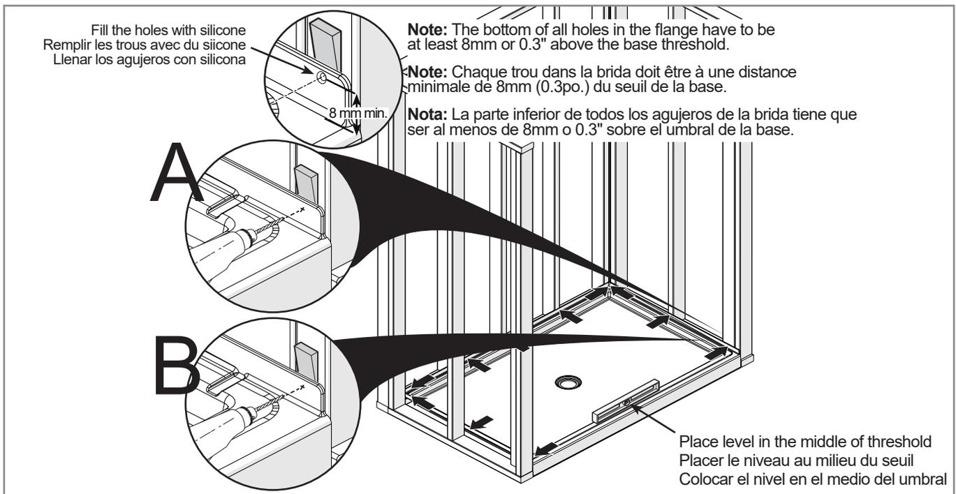
Seal the joint between the unit and the wall covering with a bead of silicone. Leave a 1" gap on the sides to work as a weep hole as shown.
