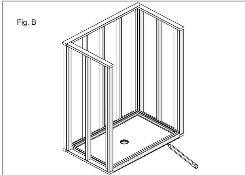
Making sure that the installation is level (position your level in the middle of the thresholds), reposition the base in place for the cement to take the form of the base perfectly while it is still wet.
