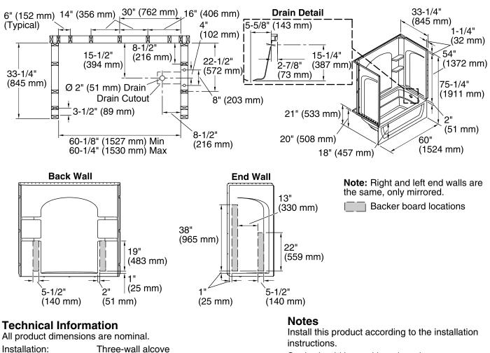
Studs should be positioned as shown.
