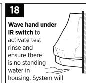
operate automatically every 72 hours from battery activation. NOTE System will pause for 2 minutes after 2 manual rinse activations.
