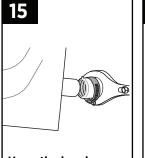
Hang the bowl inserting tailpipe into bushing, and tighten hose clamp, Install 2 lower anchor screws with washers.
