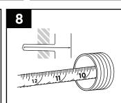
Determine the drain nipple **length** by measuring the distance between the back of the sanitary tee (or elbow) the front edge of the nipple.
