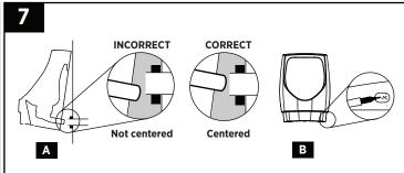
A. Hang bowl on the bracket and check tail pipe alignment, then remove the bowl and adjust the bracket as needed. Re-hang and re-check bowl alignment with the drain line. Tail pipe should align with center of drain line. B. Mark anchor holes then remove bowl without moving hanger bracket.
