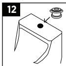
With urinal on the floor insert rubber grommet into the hole located at the top of the urinal. Be sure the larger diameter side is facing up and fully seated.
