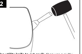
Use utility knife to cut caulk then use a putty knife and mallet to remove the bowl. Remove hanger brackets, scrape off caulk, and clean the wall. Ensure the threads on the control stop are
