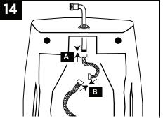
A. Securely connect the female end of the loose braided hose to the end of the supply assembly. B. Connect the male end to the braided hose on the Hybrid Jetrinse assembly on the urinal. NOTE Ensure that these connections are tight and leak-free.
