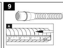
A. Find the drain nipple depth on the Tube Cutting Chart (left). Measure and mark the specified **trim length** on the insert tube at the nearest 1/4" groove.
