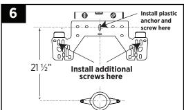
Measure and mark the rough-in if in-wall carrier is not used. Use a 5/16" masonry bit to drill hole, then install the hanger bracket with one plastic anchor and screw. Level the bracket then mark, drill and install two additional plastic anchors and screws.
