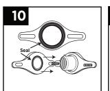
Place the seal into the flange with ribs facing out. Install the flange with washers and hex nuts, but do not over tighten.
