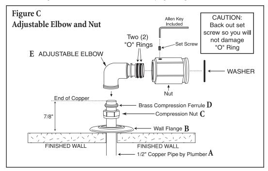
Please Note: The entire valve body must be installed over the copper pipes
