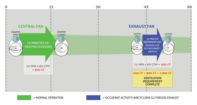
After regular heating/cooling cycles and manual occupant use of bathroom exhaust fan, ventilation requirements for the hour were met. No need for additional ventilation forced by AirCycler® g2.
