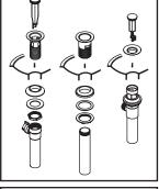
and apply Teflon tape on threaded tailpiece. Thread tailpiece to drain body. Insert flange through drain hole and attach drain body to flange from underneath the sink. b. For 50/50 type pop-up: Place a ring of plumbers putty on the bottom of the flange. Insert drain body through drain hole. Thread rubber gasket, flat washer, and lock nut onto drain body. Apply Teflon tape only on the
