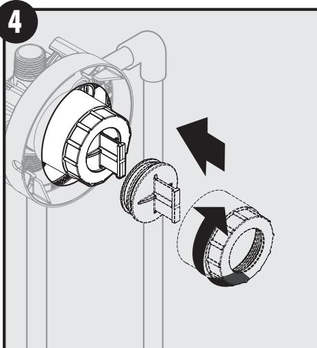
Reinstall flush plug and cap to secure the cross flow plug. Flush plug nut to be hand tight.
