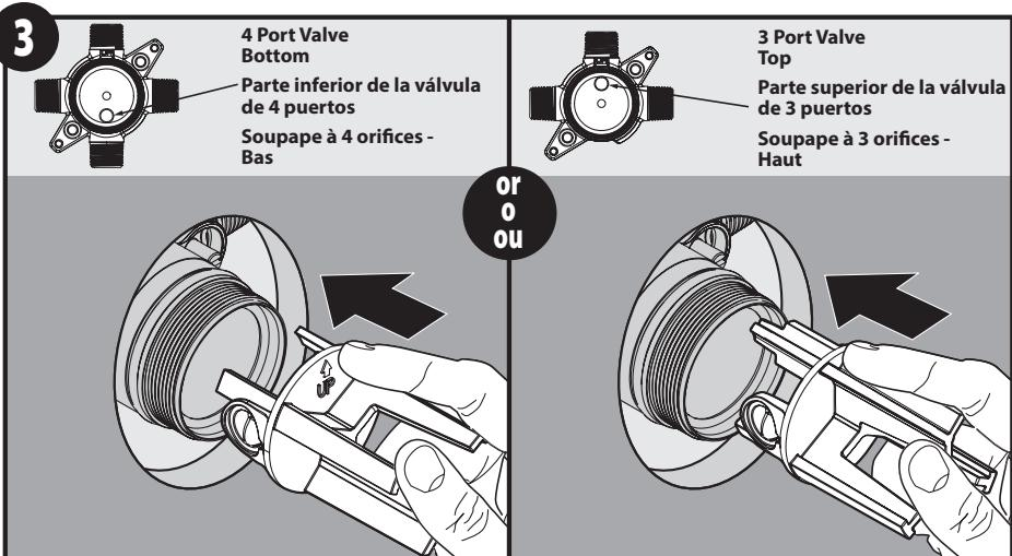
Install assembly from **Step 2** into valve, with arrow pointed up.
