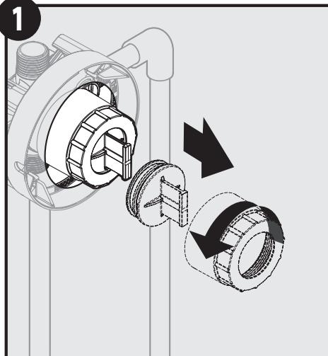
Remove flush plug nut and flush plug.
