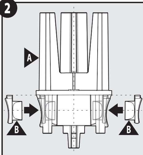
Install rubber check valves (B) into the cross flow plug (A) which are included with this kit.
