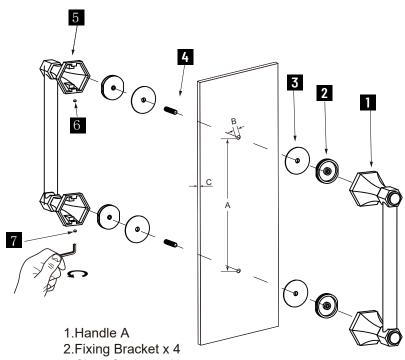
2.Fixing Bracket x 4 3.Clear Gasket x 4 4.Bolt x 2 5.Handle B 6.Set Screw M5 x 2 7.Allen Key 2.5mm x 1
