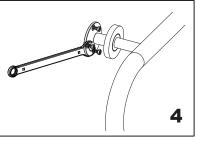
Driver bolt nut directly into holes
