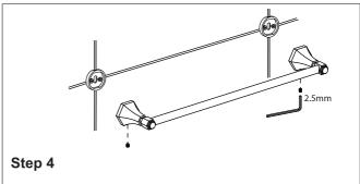
Slide the accessory onto the backing plates and tighten the set screws using Allen key provided.
