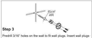
Predrill 3/16" holes on the wall to fit wall plugs. Insert wall plugs into the wall. Position backing plate flat side down over the plugs and install screws.
