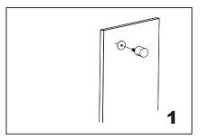
Install the knob (bolt) through the glass hole, make sure the rubber gaskets are between knob&glass.
