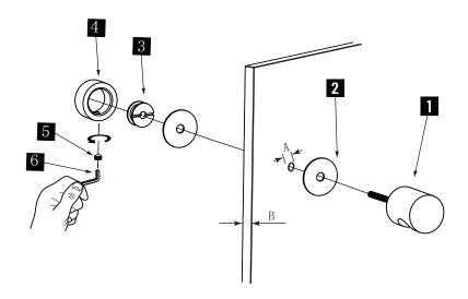
1.Knob x 1 2.Clear Gasket x 2 3.Fixing Bracket x 1 4.End Cap x 1 5.Set Screw M5 x 1 6.Allen Key 2.5mm x 1
