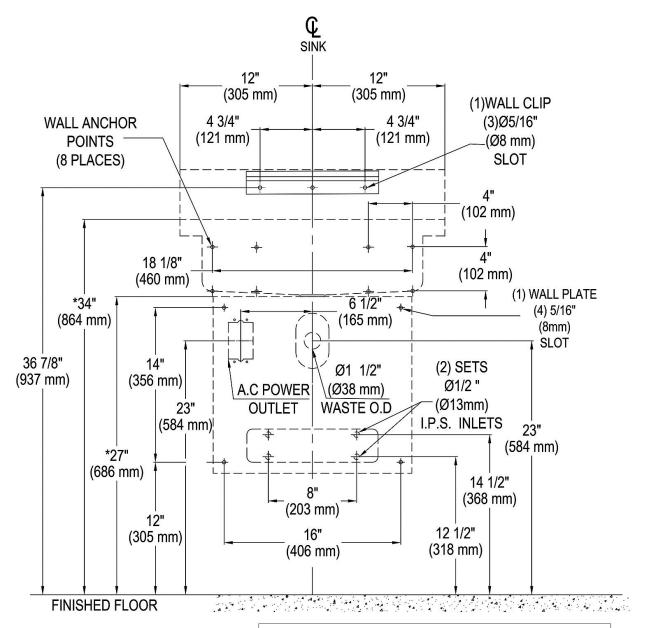
\*NOTE: ALTERING THIS DIMENSION COULD CAUSE SINK TO BECOME NON-ADA COMPLIANT
