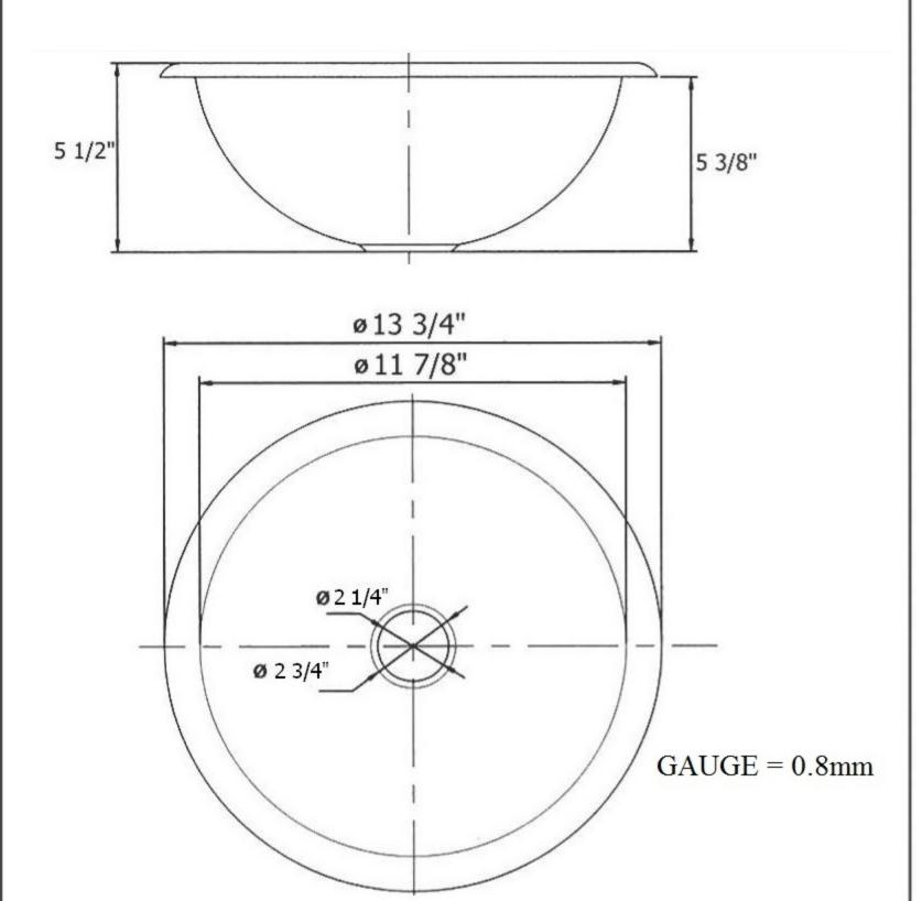
NOTE: Pre Dec. 2014-used 4520 1 1/4" Grid Strainer Dec. 2014 Now Uses 4521 1 1/2" Grid Strainer Dimensional Change Dec. 2014
