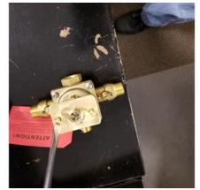
4. Take #4 bell and ensure #9 stem is inserted into the back of #4 bell as shown below left. Insert the assembly through the center of #1 mounting plate and fit it onto the rough nipple. Now finish screwing #2 slotted screws down tight to secure mounting plate to rough. (This aligns bell & stem.) Remove #4 bell & #9 stem and set aside for next step:
