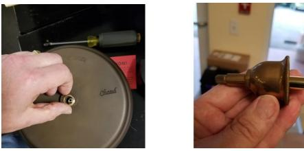
6. Install #4 bell & #9 stem into center of #3 wall plate and turn the stem fully clockwise. (Note that #4 bell & #9 stem will sit slightly above the wall plate so it can turn freely without scratching the wall plate.):
