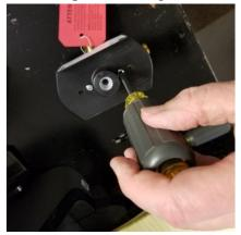
2. Remove #2 white plastic stem from rough with Phillips screwdriver and set aside:
