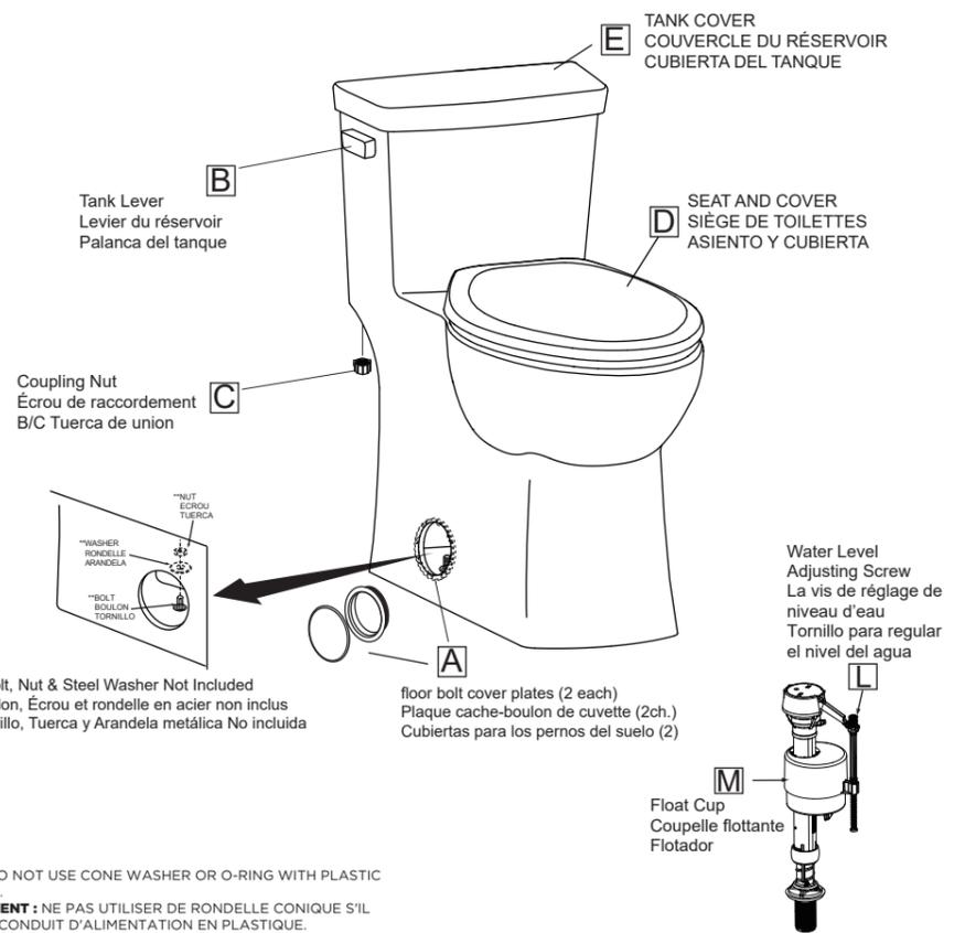
**CAUTION:** DO NOT USE CONE WASHER OR O-RING WITH PLASTIC SUPPLY LINE.
