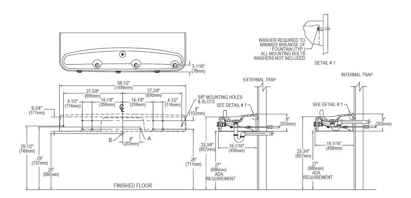
LEGEND A = 3/8" O.D. Unplated copper tube connect - shut off valve by others B = Water outlet 1-1/2" O.D. drain stub out from wall 1" (25mm)
