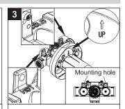
Using mounting holes secure the valve making sure the "UP" label outlet is on top. Hot should be on left, cold on right.
