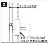
Turn off the water supplies. Install the valve so the finished wall will fit between the markers on the mud guard.
