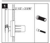
This valve is designed to fit into a wall that is 2 1/2" to 3 5/16" from finished wall to the back of the valve. If necessary, extensions can be purchased separately.
