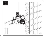
Connect top outlet with proper fittings.Note: it is suggested that you anchor all water lines.
