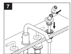
Pull black nylon or finished hose through the hand shower nipple bracket. Slide the hand shower bracket and hose guide over the hose. Secure the assembly with the thread. Note, make sure the hose does not slip under the deck.
