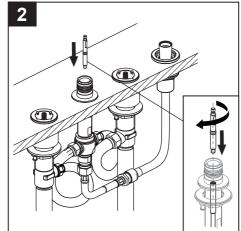
Connect the diverter rod extension to the diverter rod in the diverter spout nipple.
