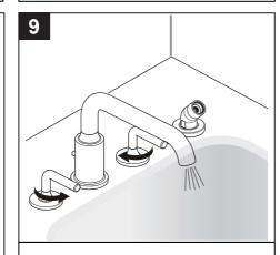
Make sure the diverter knob is in the down position. Turn the faucet handles on full for one minute to flush debris.
