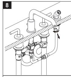
Remove the aerator with the supplied key. Turn the water supply on.
