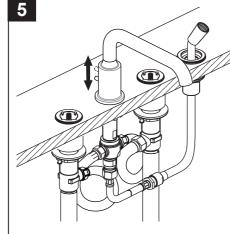
Pull the diverter rod and knob up and down to test the connection.
