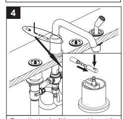
From the back of the spout insert the diverter knob into the spout and carefully place it on the diverter rod. Secure the knob with the setscrew.
