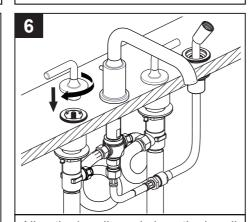
Align the handle and place the handle and escutcheon assembly onto the valve. Secure the assembly by turning the escutcheon clockwise. Repeat for the other valve.
