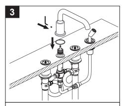
Place the spout "O" ring under the spout and install spout on spout nipple-diverter assembly. Be sure the spout is firmly resting on the deck. Secure the spout with the setscrew.
