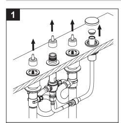
Turn the water supply off and remove the mud guards.
