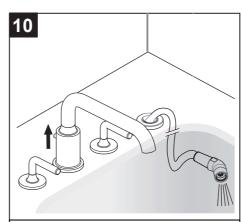
Leaving the water on, pull the hose to its farthest extension and point it into the tub. Pull the diverter knob to its top position. Flush the debris for one minute. Turn off the valves.
