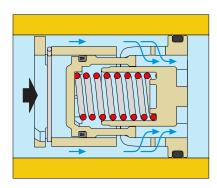
If the differential pressure is within the control range, the spring-loaded piston is positioned to give the fluid a free flow area permiting regular flow at the **nominal rate** for which the FLOWCAL is set up.
