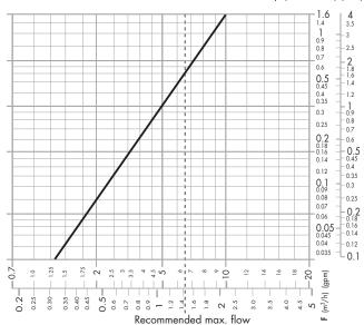
The maximum recommended speed of the fluid in the piping is 4.2 ft/sec, which is equivalent to a flow rate of 6.5 gallons per minute.
