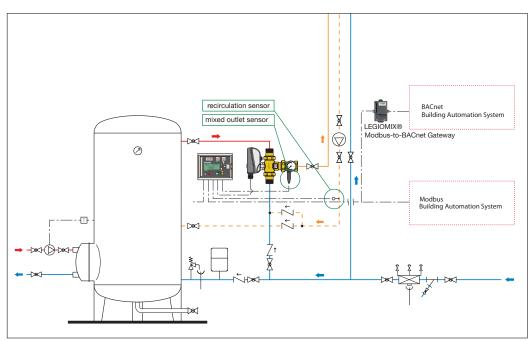
Modbus-to-BACnet gateway for remote control
