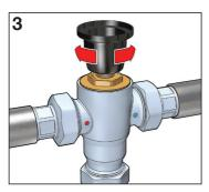
Temperature adjustment cap in place
