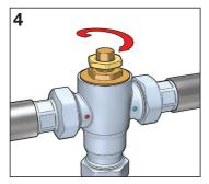
Locking adjustment spindle with locking nut
