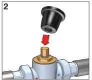
Attaching temperature adjustment cap
