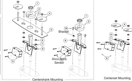
NOTICE! Sensor must be flush and parallel with the lens. Do not force or bend the bracket!
