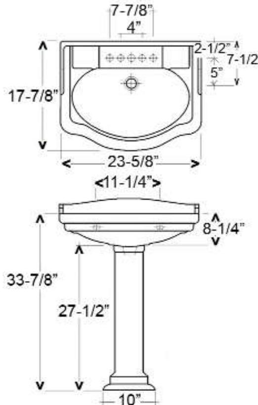
Dimensions of fixture are nominal and may vary within the range of tolerances established by ASME Standard A112.19.2-2018. Dimensions and specifications subject to change without notice.
