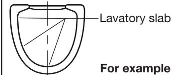
Place lavatory and pedestal into installed position. Level and square the lavatory and pedestal
