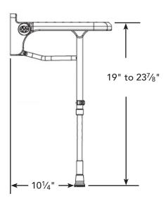
Seat width overall:  $18\frac{1}{4}$ " Seat depth overall:  $15\frac{1}{4}$ " Wall to front edge of seat
